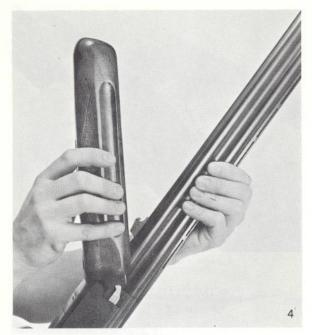
To attach the forearm to the barrels, hold the gun at the barrels with the butt of the stock resting on your thigh with the trigger guard up. Engage the rear of the forearm at the front of the receiver and pivot it into place, then snap the forearm release closed. (Fig. 4)
