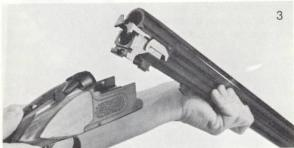
To attach the barrels to the receiver, grasp the receiver at the pistol grip and tuck the butt section between your body and arm just above the waist. Grasp the barrels with the other hand above the forearm lug. (Fig. 3) Hook the barrel lug recess (A) over the hinge-pin (G, Fig. 2) in the front of the receiver, and pivot the rear of the barrels into the receiver by lifting sharply on the barrels.
