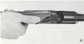
the forearm away from the barrels. (Fig. 5) To remove the barrels, grasp the stock at the pistol grip and place the butt section under your arm against your body. Grasp the barrels in the other hand. Push the top lever to the right (Fig. 6) and pivot the barrels down until they disengage from the receiver. (Fig.7)
