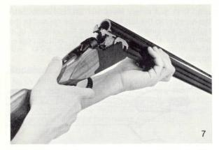
For storage, the forearm may be reattached to the barrels when disassembled. Place the rear of the forearm in the position it would normally be for assembly and pivot toward the barrels and lock in place. Snap the release lever closed.
