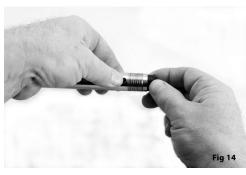
3. With your other hand grasp the protruding portion of the magazine spring retainer and slide the magazine spring retainer forward until it clears the magazine tube. Use caution as the magazine spring retainer is under spring tension from the magazine spring.
