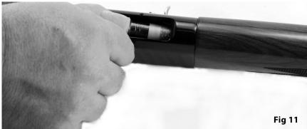
To Feed a Shell from the Magazine into the Chamber
