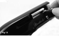
The piston will work only if the large outside diameter of the piston is placed onto the magazine tube first.
