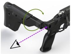
**3.** Using a ball head 7/32" allen wrench undo the screw revealed behind the hinge mechanism.
